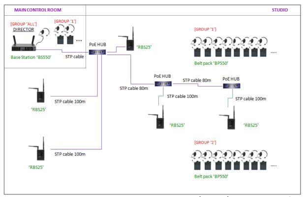
[Figure 12] System usage example
